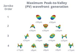
RMS residual wavefront error : max  $0.02\mu m$  (generation of Zernike mode of the order <5 with amplitude set at 20% of the total dynamic range)
